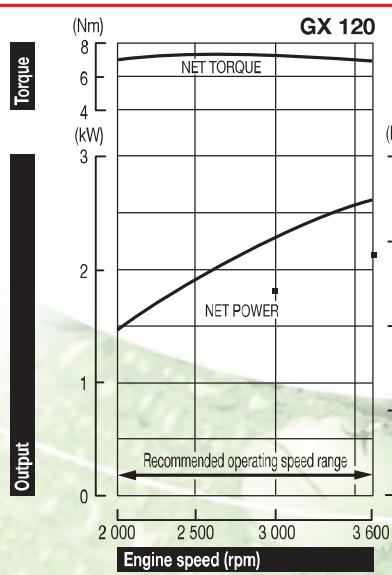
The power rating of the engine indicated in this document is the net power tested on a production engine for the engine model and measured in accordance with SAE J1349 at a specified rpm. Mass production engines may vary from this value. Actual power output for the engine installed in the final machine will vary depending on numerous factors, including the operating speed of the engine in application, environmental conditions, maintenance, and other variables.
